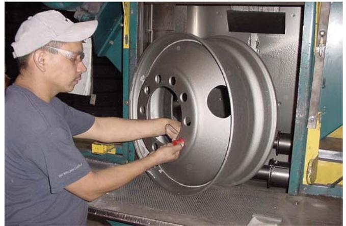
For grade level 4 through 9, we can refinish these wheels using our state-of-the-art Powder Coating systems. During the powder coating process, the wheel is shot blasted to a bare metal surface. The wheel is then inspected for cracks, worn bolt holes and defects in the rim flange area.
