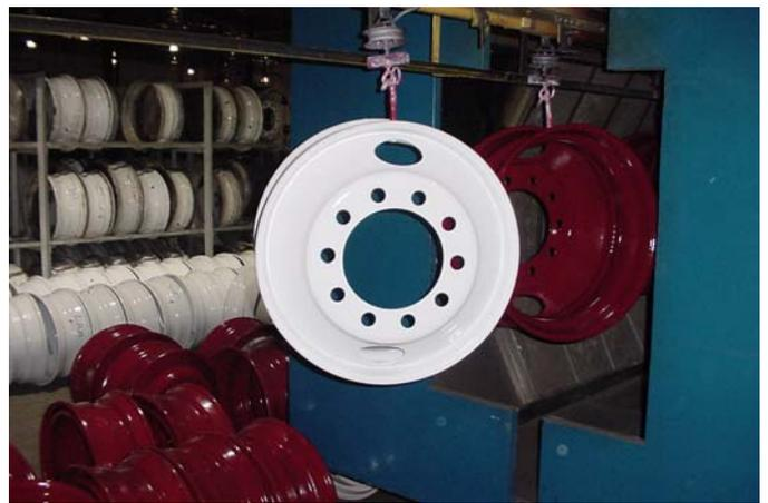
The paint is cured using our state-of-the-art "Gas Catalyst Infrared" ovens to evenly cure the powder to the wheel. Our ISO certified painting systems deliver high quality, time after time.
