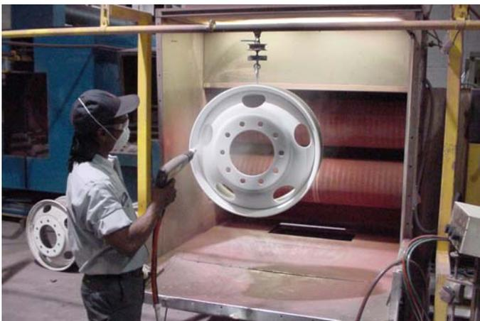
We then apply a uniform coating of high quality polyester based powder paint, which is then cured to the wheel in our Infrared oven.
