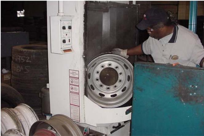
For wheels that exceed the fleet's minimum appearance standards based on our grading system, STI will wash or refinish the wheels. If the fleet's wheel is graded a level 1 through-3, we can wash this wheel and safely return it to service.
